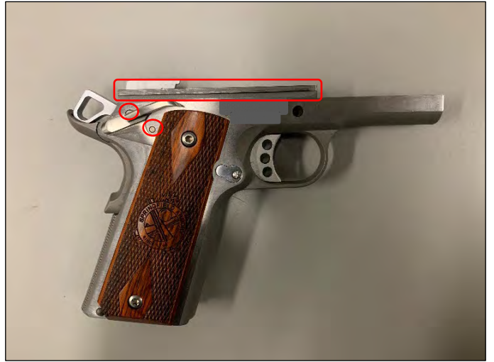
The machining of the Hammer Pivot Pin Hole, Sear Pivot Pin Hole, and Slide Rails on this 1911 style handgun frame has been completed.
