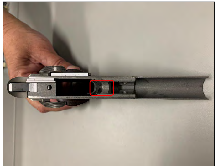
The machining of the Barrel Seat and Barrel Lug areas on this 1911 style handgun frame has been completed.
