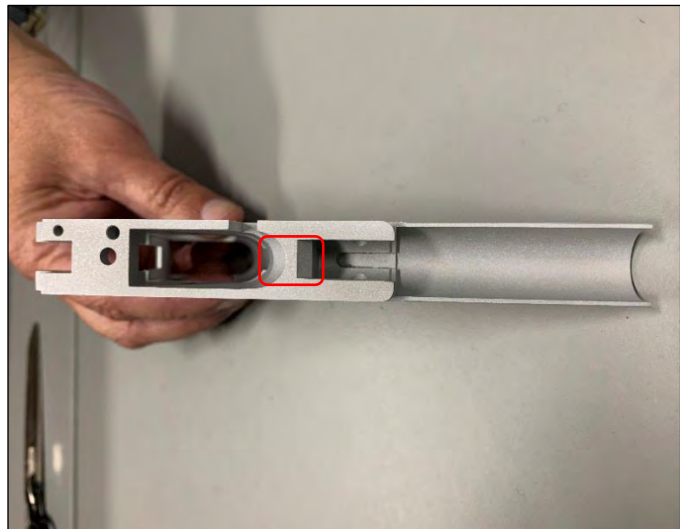
The machining that would be necessary to give this unfinished 1911 style handgun frame a Barrel Seat or Barrel Lug area has not been completed.
