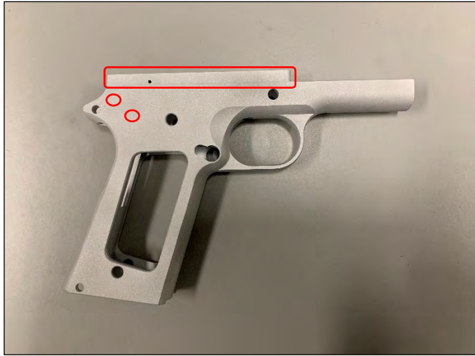
The machining that would be necessary to give this unfinished 1911 style handgun frame a Hammer Pivot Pin Hole, Sear Pivot Pin Hole, or Slide Rails has not been completed.
